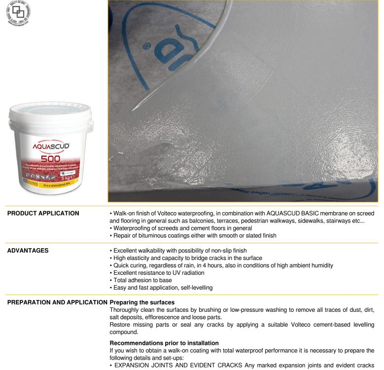
• EXPANSION JOINTS AND EVIDENT CHACKS Any marked expansion joints and evident cracks found on the surface must be covered with GARVO joint cover strip (see relevant technical data sheet), for which it is recommended to prepare a lowered application site of approximately 2-3 mm by means of shaping during the casting stages of the cement-based surface, or subsequent milling, in order to allow flush application of the tape
